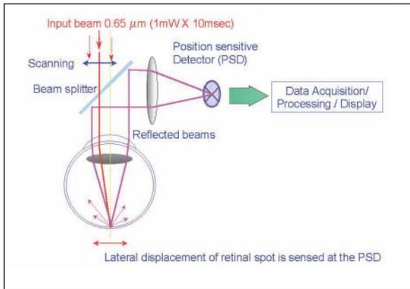
Figure 1. Schematic diagram of Tracey.
